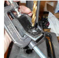
Drill bottom plate through holes in bracket - clamp compresses rubber to get metal to metal contact
