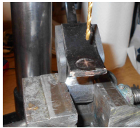
Drilling pilot hole
